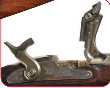
The Model 1865 rifle (top) initiated Erskine Allin's innovative hinged-breechblock (inset) concept. Rock Island Auctions
